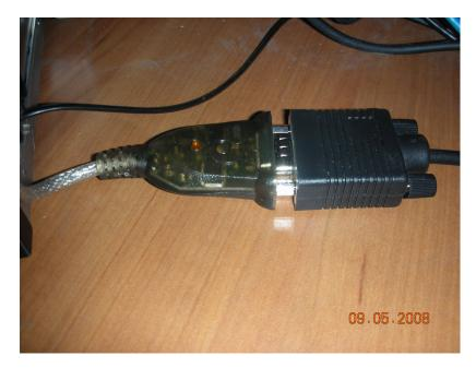
The USB to Serial adapter used is like the one on the web page at <u>http://www.iogear.com/product/GUC232A/</u>
