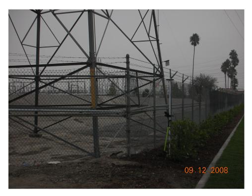
It was important to understand the potential for both fixed solution performance and accuracy. Geodetic survey control monuments established by the National Geodetic Survey would be used to evaluate the accuracy at various ranges. NGS control points were selected because they represent a national standard.
