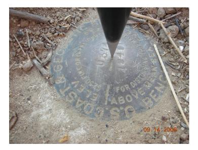
FAULT L (PID: DS3746) is a NGS GPS control point with network accuracy estimates computed from what is on the data sheet. The network accuracy is for the ellipsoid height. The NAVD88 elevation was computed from the ellipsoid height and the Geoid height published on the data sheet. FAULT L is 10.6 miles southeast of the base.
