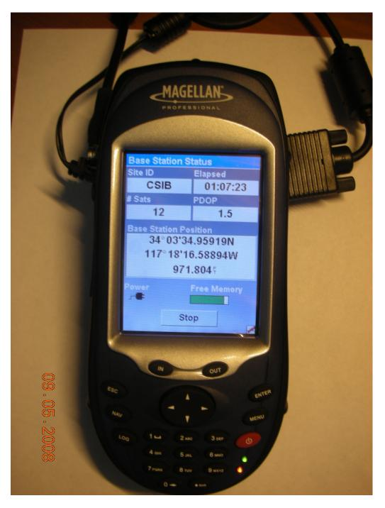
A ProMark3 with cables connected is set to broadcast RTK corrections using the Surveying program.
