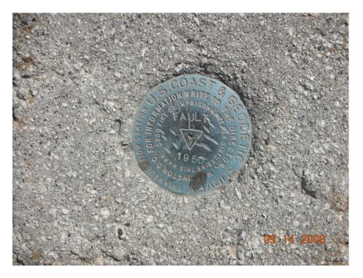
Look at this in very old fashioned terms: The measurement gives a closing error of 0.23 feet at a distance of 55,901.66 feet for an accuracy ratio of 1:243,000. That may have little to do with modern methods of accuracy determination but it is a way that makes sense to a dirt surveyor who is nearly as old as that brass cap. FAULT L was not part of the survey that determined the coordinates for the base station.
