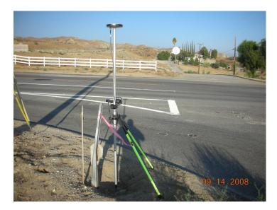
U 374 (PID: DX2564) is a NGS first order bench mark with a published elevation of 1979.91 feet. It is located about eleven miles southeast of the ProMark3 base station. There are no published horizontal coordinates to use for a comparison but many people say the elevation is the hard part of GPS accuracy. This project includes several RTK shots on U 374 during the first visit and again on repeat visits on different days.
